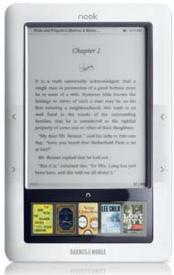
**Battery Life:** The Nook has a battery life of up to 10 days before recharging, and the rechargeable battery is replaceable by the user. The Nook Color has up to 8 hours of use before recharging, and the rechargeable battery is not replaceable.
